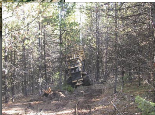
Figure 8. (Right) All Surface Vehicle (ASV) with slash buster head thinning young Western Larch stand.
