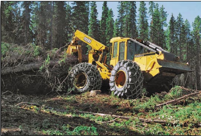
Figure 9. A rubber-tired skidder removing commercial trees from the woods.
