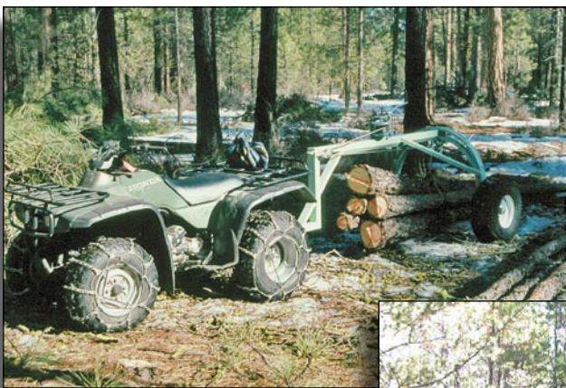
Figure 7. (Above) ATV with “log arch”. Example of light duty harvesting equipment for smaller diameter logs.
