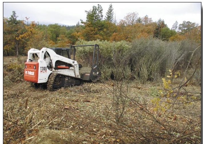
Figure 4. Brush mulcher treating manzanita and wedgeleaf ceanothus brushfield, SW Oregon. Cutting head is mounted on “Bobcat.” Efficiently cuts material up to 4” diameter.
