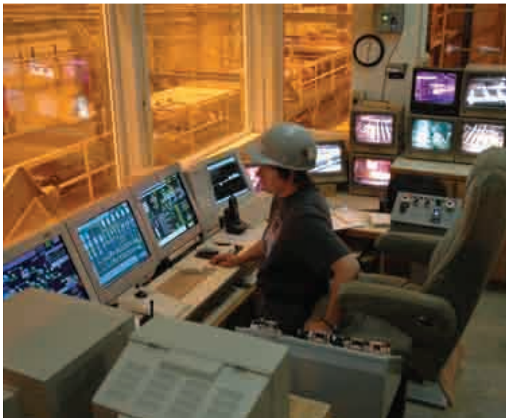
Much of the operations of plants like Boise Cascade's particleboard facility are monitored and controlled from booths like this that are situated in visual proximity to the lines. The real operation of these massive manufacturing lines takes place in these rooms, where the positive logic control that comes from sophisticated computers ensures that each action is coordinated with all the others. Here is the place where operators can identify problems on the line, and often coordinate repairs as well.
