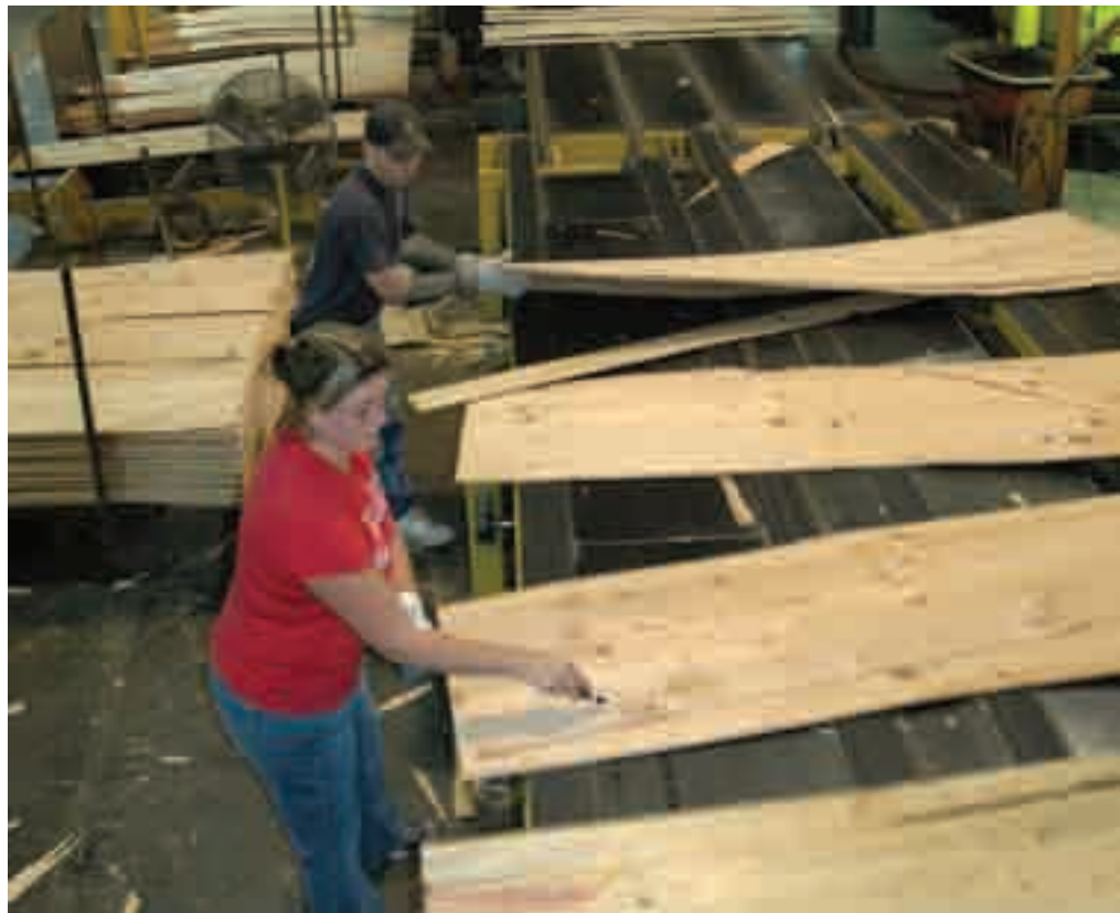
Wood is a natural material, and because each tree is unique in terms of branch structure, ring density and other factors, converting it into a consistent, high-quality product requires skill and experience. Here expert graders quickly assess each piece of material as it moves down the line and assign it a mark to indicate its characteristics. This process ensures that consumers will be able to buy wood products appropriate to their intended use.
